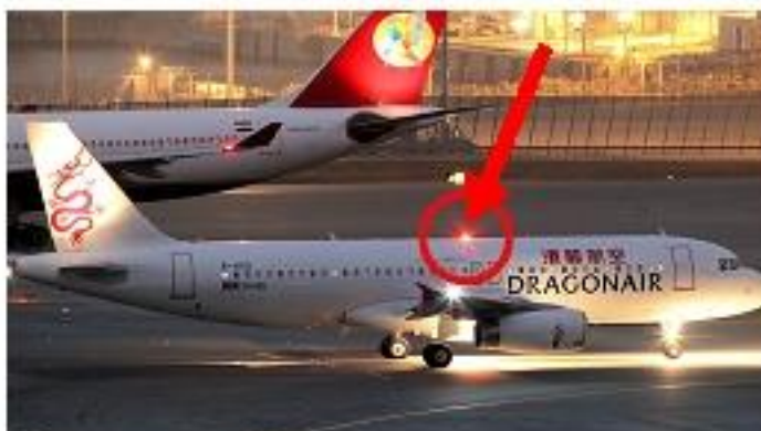
Photo of aircraft with beacon light flashing above the aircraft
